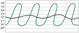
Typical Single-Stage Operation - Low-Stage Operation of a Two-Stage Unit -
